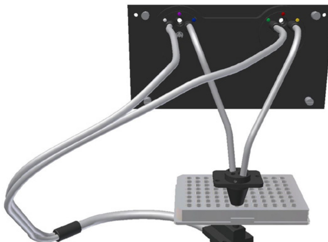
Figure 17: Principle drawing of top and bottom optics
