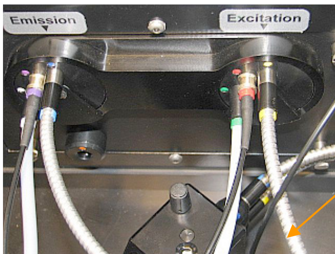
Figure 23: Final look of the installed TRF optic head and light guides.
